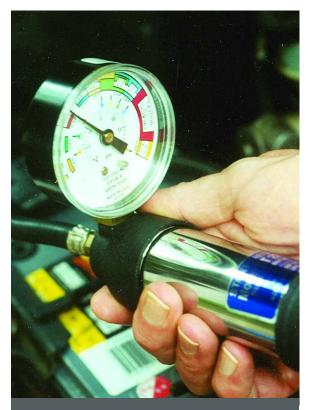
If a leak isn't obvious, a pressure tester is still the first thing to use to locate it. Pump up the system, then look around under the hood with a good light and listen carefully for hissing.
