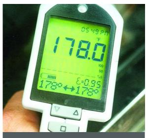
After you get a basic understanding of heat flow from using a non-contact infrared pyrometer on normal systems, it can help you locate clogs and hot spots.
