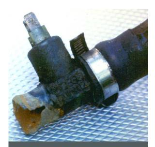
Neglected coolant maintenance, or the use of the wrong anti-freeze, will not only lead to clogging and inefficient heat transfer, but also to component erosion/corrosion and leaks at connections and joints.
