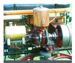
The engine of the 1886 Benz Patent Motorwagen was water cooled, and that copper jug on top served as the heat exchanger. It wasn't pressurized, however – the water just boiled off.
