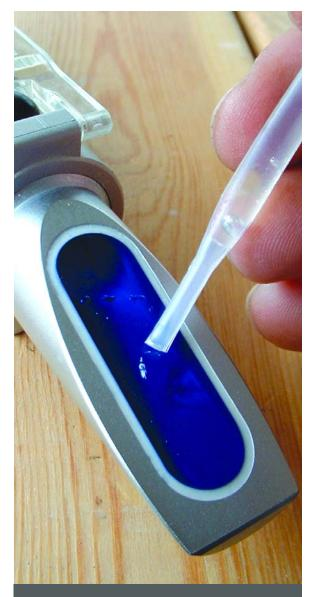
The hydrometer has been the standard tool for gauging the percentage of anti-freeze in the coolant blend for decades, but a refractometer is far more accurate and dependable.
