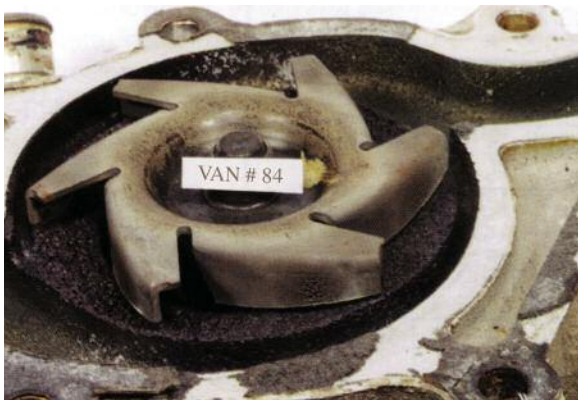
This coolant pump chamber was pockmarked by cavitation erosion-corrosion, which would eventually reduce performance of the pump.
