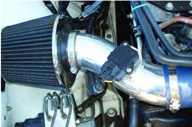
Fooling around with any tuner tricks, such as installing a low-restriction air cleaner, can easily cause OBD II to set codes because it interferes with what the ECM expects to see. This particular item, however, was engineered to place the MAF in such a position that it duplicates the original signal.
