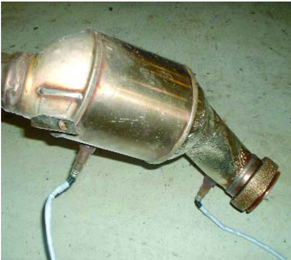
Here, you can see the positions of the upstream and downstream oxygen sensors required by OBD II. This is from a late-model Mercedes-Benz V12.
