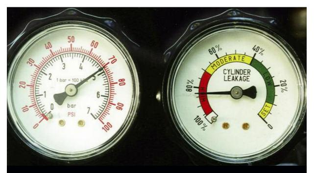
Another excellent troubleshooting procedure is the cylinder leak-down test. The gauge set lets you know what percentage of the pressure being pumped into the cylinder is escaping.
