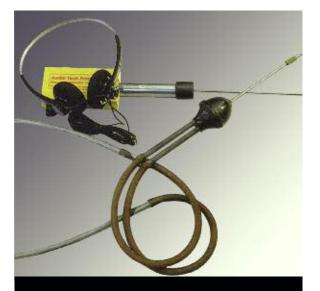
Whether the surgical tubing and diaphragm type, or one of the new electronic amplified versions, a mechanic's stethoscope is about as indispensable as it gets where nailing down noises is concerned.
