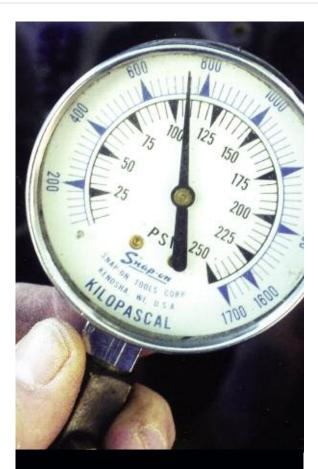
There's still nothing that can give you such a good inside picture of the pressure tightness of that cylinder than the traditional dry/wet compression test. But don't just look at the max reading. Instead, observe how the needle jumps with each of four impulses.
