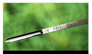
What's in the crankcase, anyway? Either too thick or too thin is a big problem. Think gasoline contamination (in the days of carburetors, we used to try to light the dipstick), or lack of maintenance that turns motor oil into tar. Your oil pressure readings will vary accordingly.
