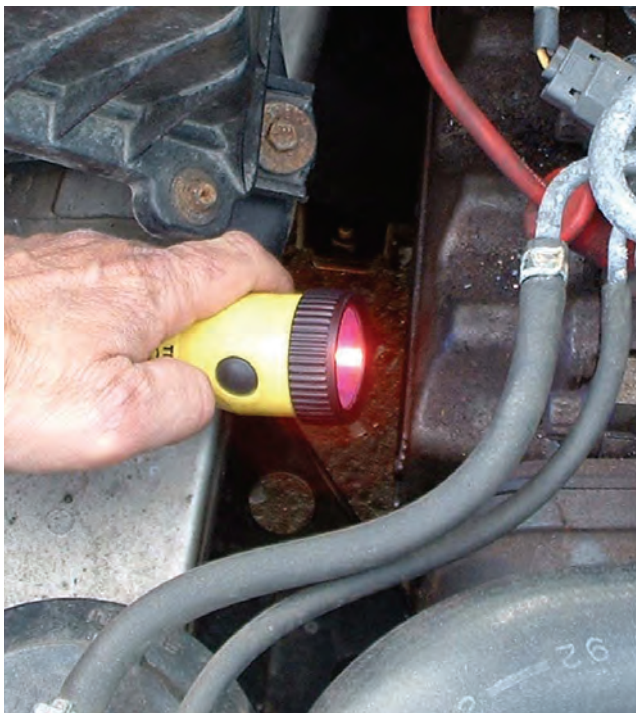
While pressure testing is probably your first diagnostic choice, nothing beats UV for zeroing-in on those sneaky leaks.
