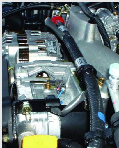
Fortunately, late-model Subaru vehicles have the A/C compressor at the top of the engine for easy access. Note also the convenient high-side service port.
