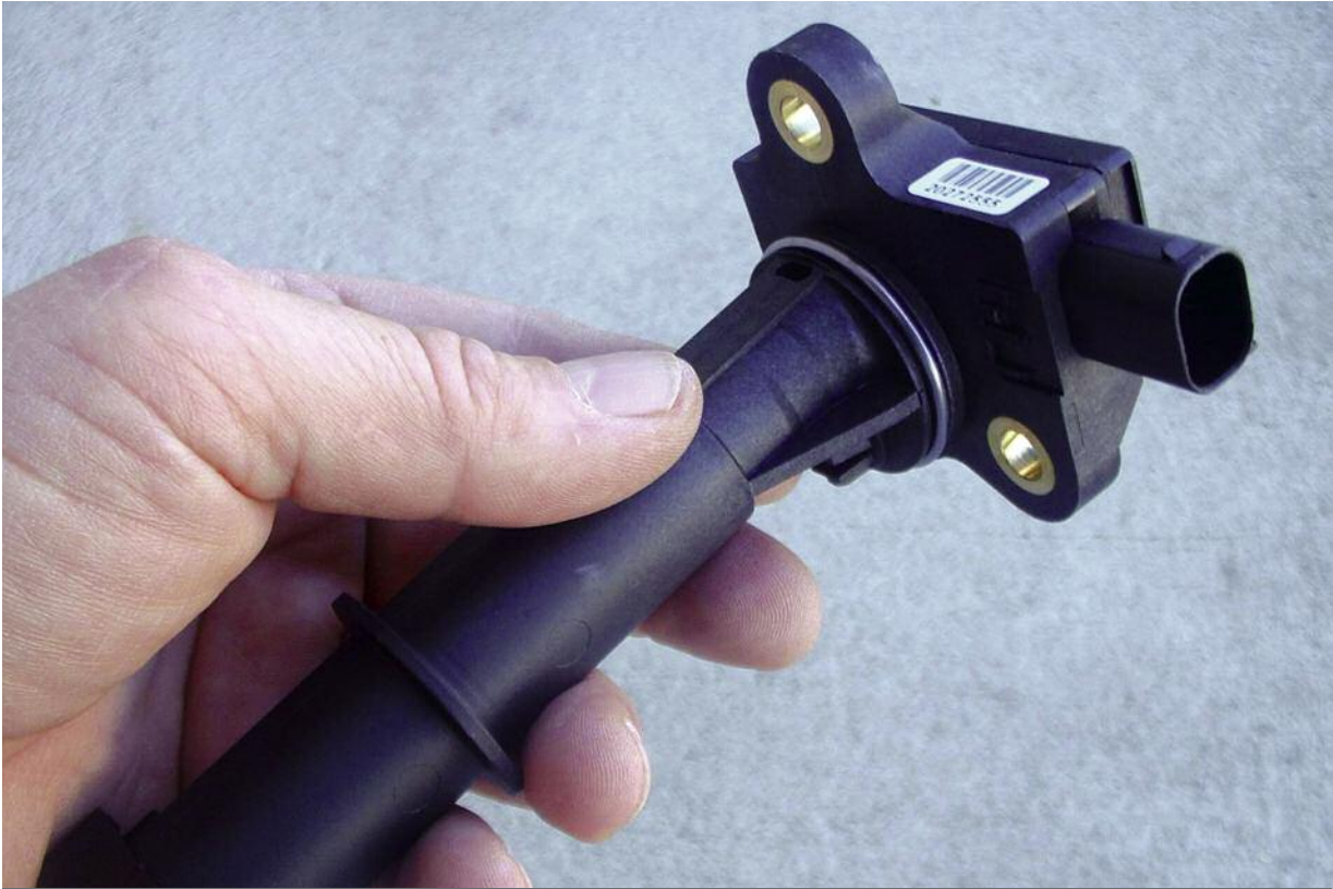
This sophisticated dielectric sensor resides in the oil pan and actually has the ability to report on the types and amounts of contaminants in the engine oil. This input goes into the electronic hopper with other info so that the computer can calculate the optimum oil/filter change interval.
