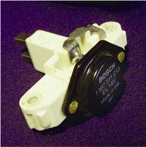
The solid-state voltage regulator is integral with the assembly that holds the carbon brushes.
