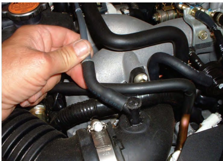
Below: Not only holes in the intake duct itself, but any vac leak in a hose that connects to it can cause the false air problem.
