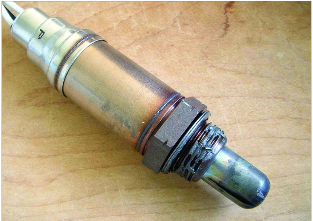
A customer who's fond of fording streams may show up at your door with the Check Engine lamp on. If you get a code 32, the oxygen sensor was probably flooded with water. Simply clear the code and the car will be good to go.
