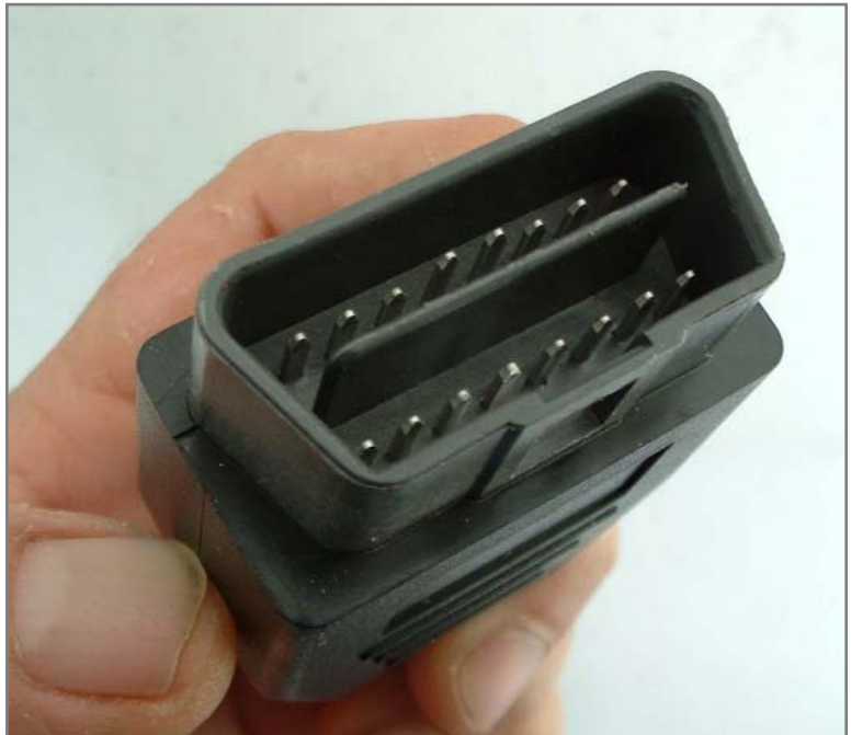
The standardized OBD II connector showed up on Subaru vehicles in 1995, and assured that not only the terrific Select Monitor, but also aftermarket scan tools could be used for diagnosis of electronic engine management problems.
