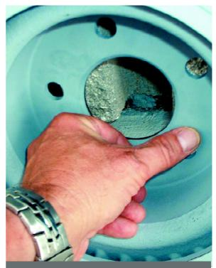
If you buy new O.E. discs, you won't have to worry about getting the mounting surface perfectly clean. The hub is a different story, however. Take your time removing all corrosion so that the rotor will run as true as possible.
