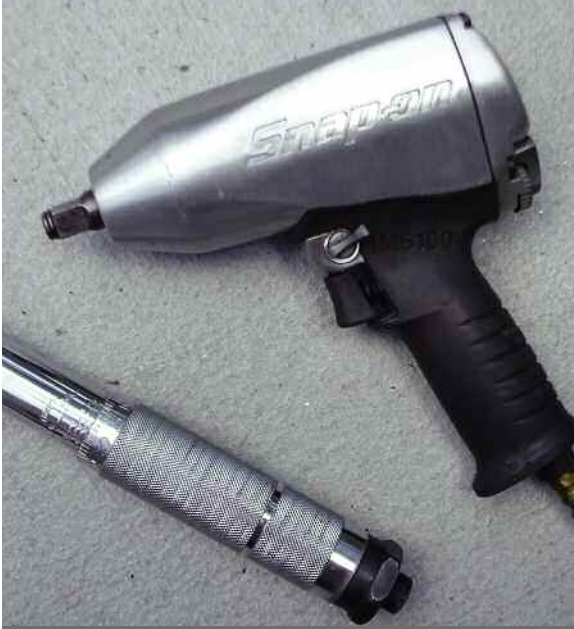
For lugs, nix on the 1/2-inch impact, and affirmative on the torque wrench.
