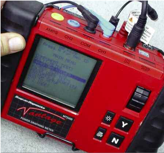
You can use a graphing multi-meter to observe the waveform the pump's motor is generating.
