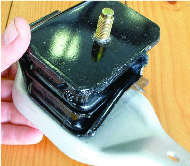
Another popular area that is unlikely to expose you to any risks is motor and transmission mounts, and “dog bone” links (called “Pitching Stopper Rods” in the catalog). The rubber in the SPT items is on the order of 10 times harder than stock, which minimizes engine and trans movement when you’re driving vigorously. This improves shifting and gives the whole vehicle a tauter, firmer personality. Once again, the risk of any liability is low.
