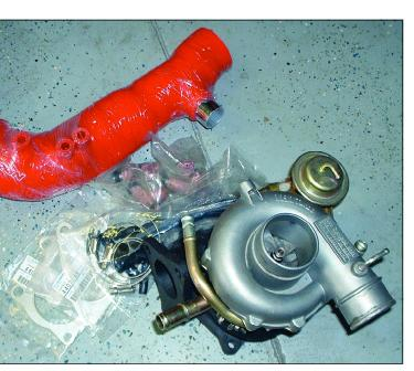
**Above:** Substituting a higher-than-stock volume turbo is one of the main ways Subatuners get those incredible horsepower numbers. Of course, other adjustments must be made to make sure sufficient fuel is supplied to make a burnable blend with all that extra air.
