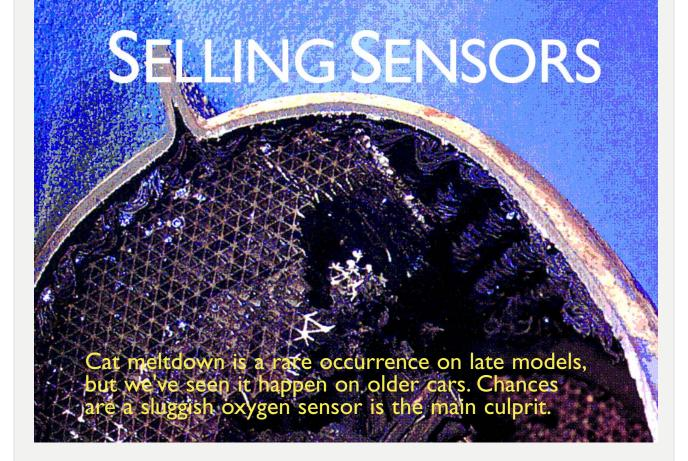
All of us in auto service know that the mixture monitor enables the engine management computer to maintain stoichiometry. That not only reduces fuel consumption and combats air pollution directly, it also allows the three-way cat to do its job of reducing NOx to harmless nitrogen and oxygen.
