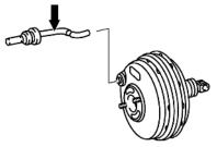
2. Replace the existing crankcase vent hose between the oil separator and the air filter housing (Figure 2) with the modified crankcase vent hose (part number A 111 018 33 82 for Model 170.447 and A 111 018 31 82 for Model 202.024), and connect it to the venturi on the brake booster hose.
