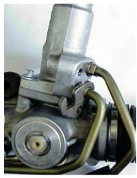
If you encounter leakage at the steering rack connection in the above models, the cause may be damage to the sealing ring of the hydraulic lines. In such instances, replacement of the rack will not resolve the situation. Instead, replace the
