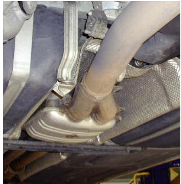
Here's a typical BMW saddle tank, which straddles the driveshaft and exhaust pipe.
