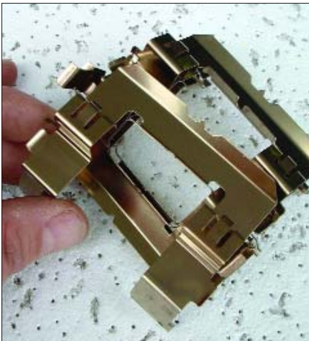
The finish quality of the caliper wear inserts from a genuine Subaru pad set speaks for itself.
