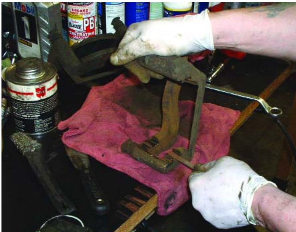
Taking the time to clean up the contact areas of the caliper and its mounting bracket will help prevent dragging and uneven wear.
