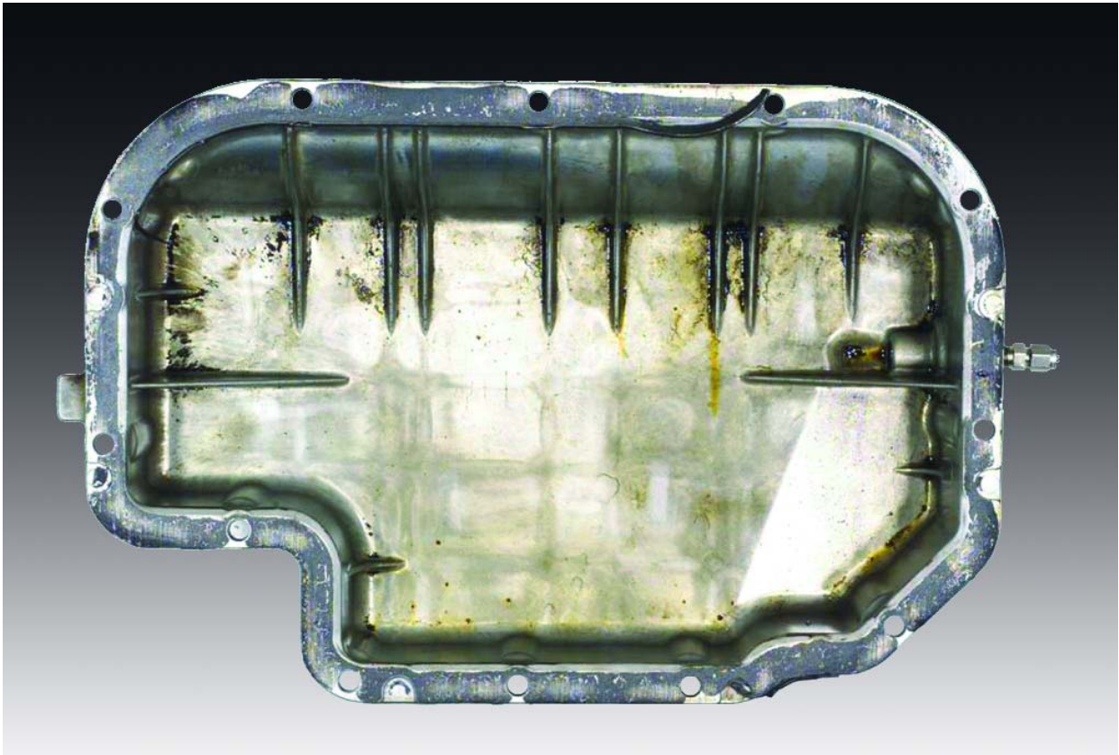
After more than 210,000 miles, this oil pan from a Mercedes E320 shows virtually no sludge. Synthetic oil was used exclusively, with 15,000 mile oil and approved filter change intervals (courtesy ExxonMobil).
