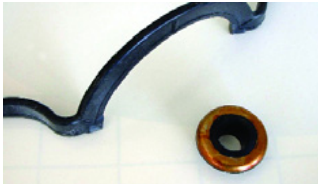
If a valve cover leak occurs, make sure you replace the little bolt seals too.
