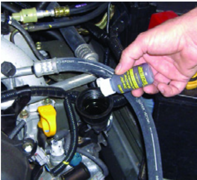
A crankcase dye and a good UV light will help you track down the most mysterious leaks.
