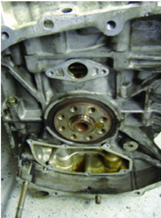
With rear crankshaft seals, direct inspection is difficult while the engine is in the car, so you've got to use some logical thinking.
