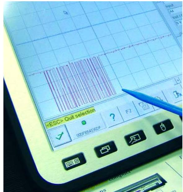
*The digital oscilloscope display on the Compact<sup>3</sup>. This is the "known good" pattern, which you compare with the live pattern that would be displayed in the space above.*
