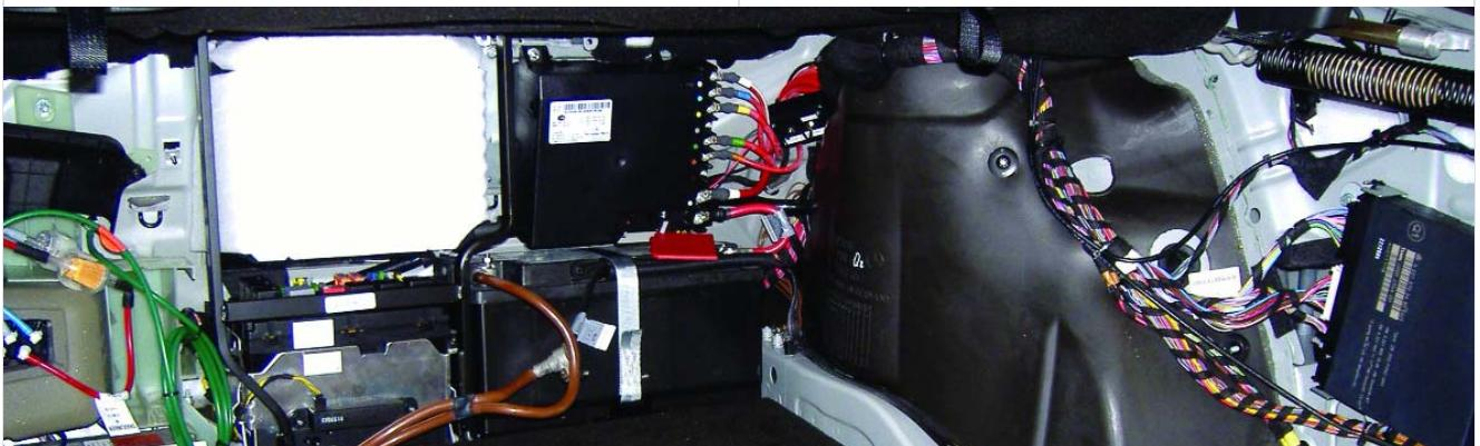
*With the trunk panels removed, you can get an idea of just some of the complex electronics on board a late-model Mercedes-Benz. Sooner or later, you'll have to diagnose these high-tech systems.*
