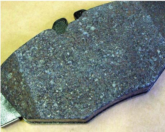
The color variations across the front of this Mercedes-Benz brake pad are caused by the different materials blended together to create the pad.
