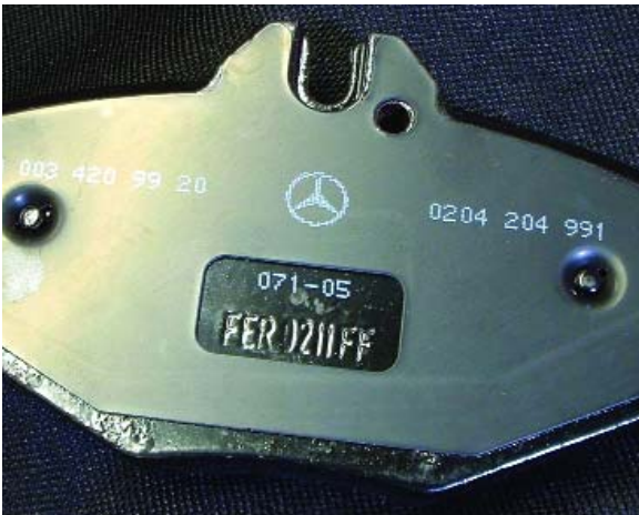
The three-point star logo and the part number on the metal backing plate show this is an authentic Mercedes-Benz replacement brake pad.
