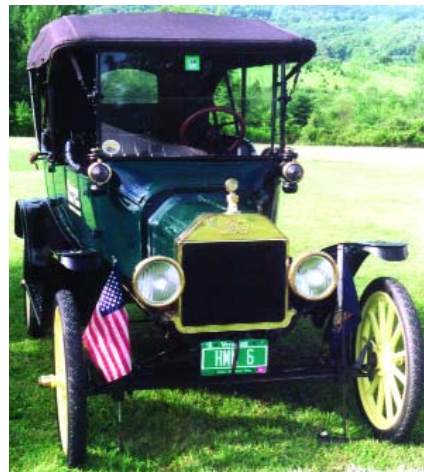
Believe it or not, the Model T got along without a water pump. The thermo-siphon principle more or less circulated the coolant.
