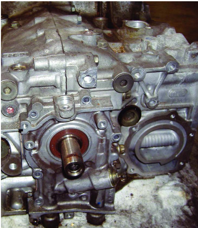
Looking into the water pump cavity, you can see that the Subaru engineers placed the pump as low as possible in the engine.
