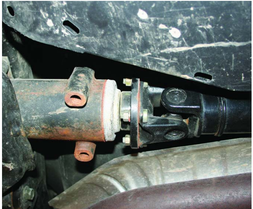
Don't forget to check the propeller shaft connector for excessive play. It can be a source of underbody vibration.
