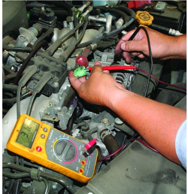
A good quality multi-function digital multi-meter (DMM) is essential for diagnosing electrical problems. Be sure to learn how to use all of its features.
