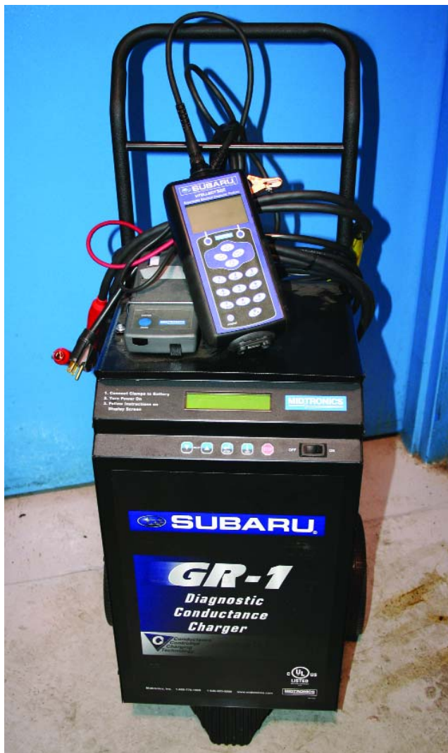
A new conductance-based diagnostics battery charger can provide quick, accurate battery testing and charging.
