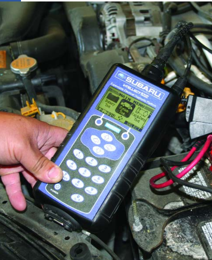
New electrical system analyzers, such as the Midtronics inTELLECT EXP-1000, have made diagnosing electric system problems much easier.
