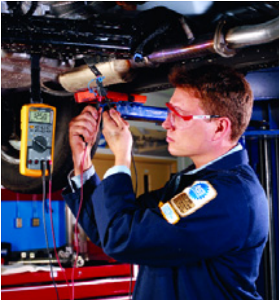
A good quality digital multimeter (or, DMM) is essential for any electrical testing (courtesy Fluke).
