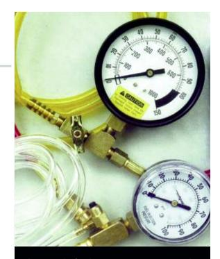
A good fuel pressure gauge is absolutely essential to any auto service operation. Many misdiagnoses have been caused by inaccurate gauges.
