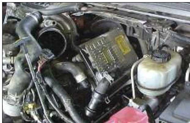
The FICM is tucked in by the firewall on this F-150.
