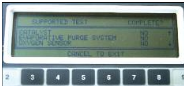
A non-continuous monitor, on the other hand, may read either "Yes" or "No" depending on whether or not it has run and completed.
