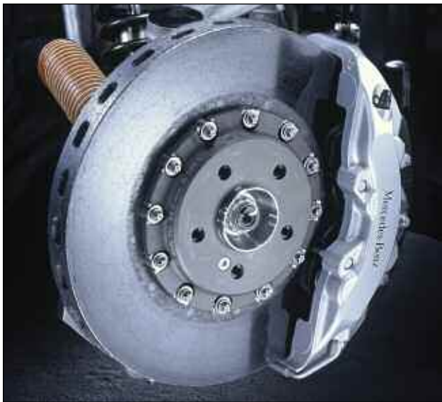
It's not likely that you'll be machining futuristic discs like this fiber-reinforced ceramic composite SLR McLaren specimen [courtesy Mercedes-Benz].
