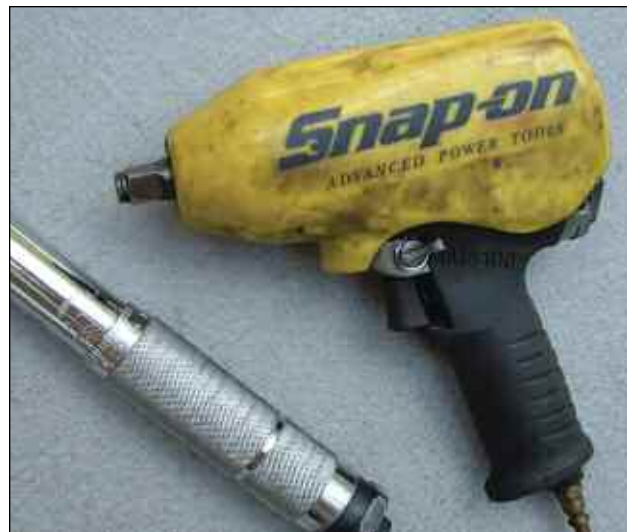
As we hope you're aware by now, you can keep from causing runout problems by always tightening lugs with a torque wrench instead of your thermonuclear impact gun. Use the proper pattern, please.
