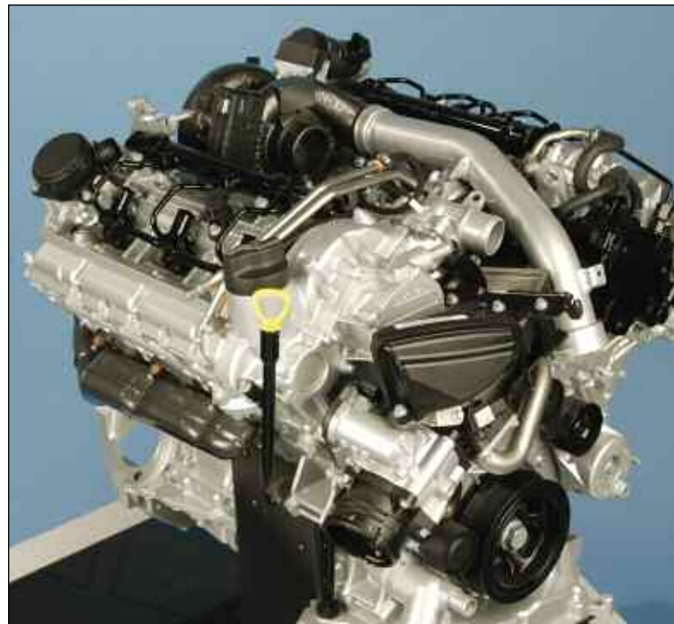
The Bosch Common Rail System (CRS) incorporates an integrated piezo-actuated injector to supply multiple sprays during compression for more complete combustion and better efficiency (courtesy Robert Bosch).
