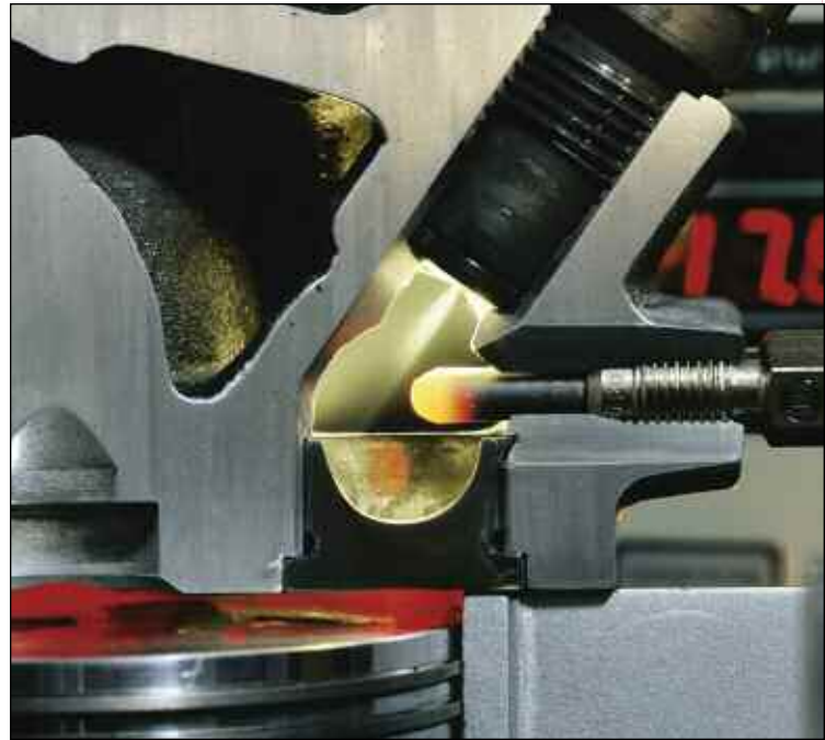
Indirect injection is a process whereby the fuel is injected into a pre-chamber and ignited. Combustion then spreads to the cylinder for the main combustion event (courtesy Robert Bosch).
