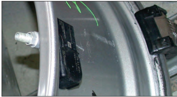
It would be pretty easy to snap off that sensor while using an old-fashioned tire machine, which will cost you maybe $125. Note the claw that grips the rim on this modern table-type machine.
