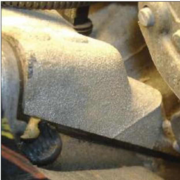
This Rendezvous 3.4L had its intake gaskets replaced twice in 35,000 miles, each time with a newer generation design. At 70K, it seems to be holding, but how much does the retrofit from DEX-COOL to conventional antifreeze have to do with it? Note extruded RTV.
