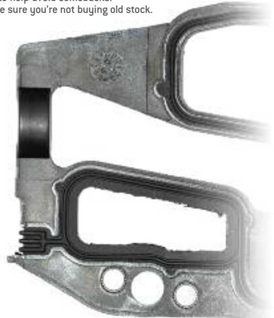
Ditto for the latest version of the 3.4L gasket. Note the barrier outlining the seal that prevents contact with the coolant.
