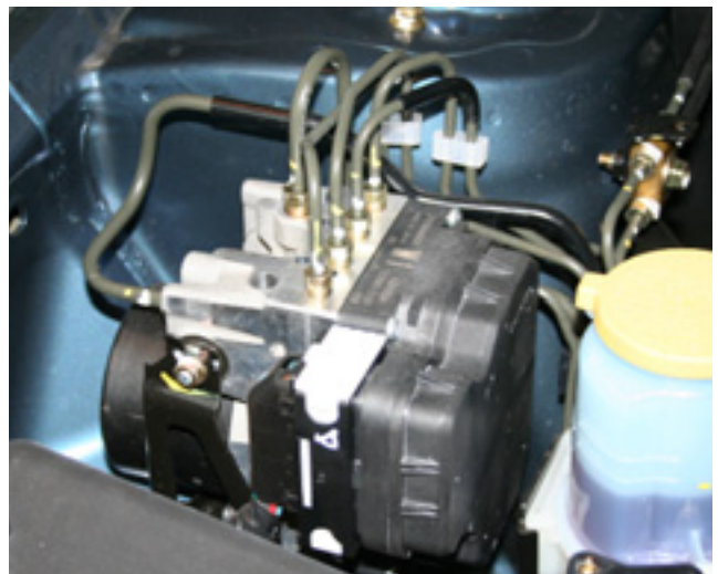
The VDC control module (VDCCM) is located on the passenger side of the engine compartment.
