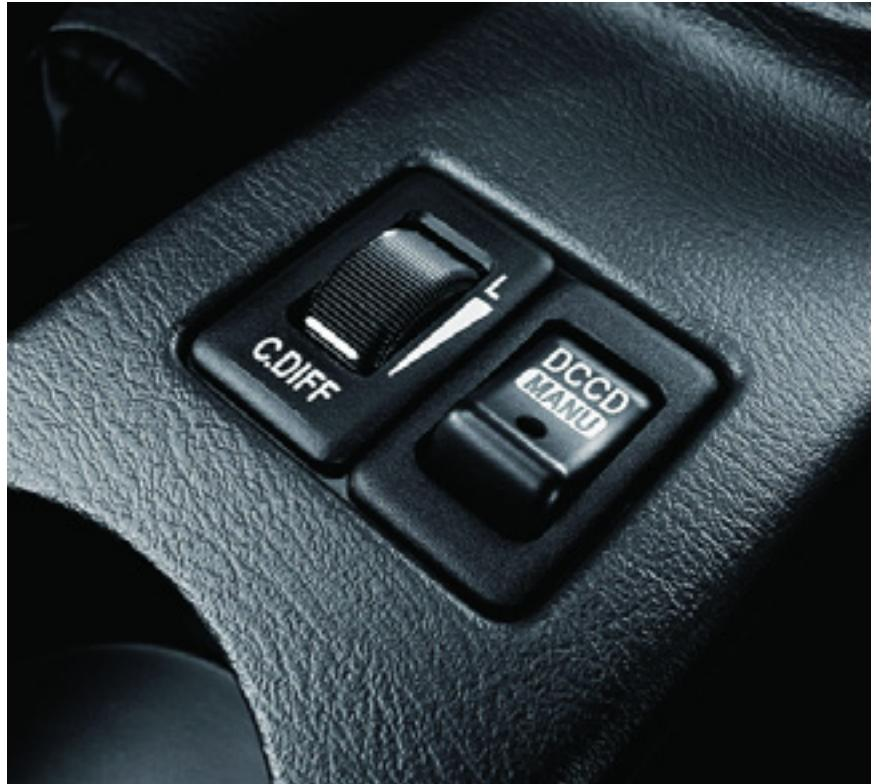
*The Impreza WRX STI uses Driver Controlled Center Differential (DCCD) to switch the All-Wheel Drive system between automatic and manual modes. Seen here, the controls allow the driver to select the mode and the level of center differential locking.*
