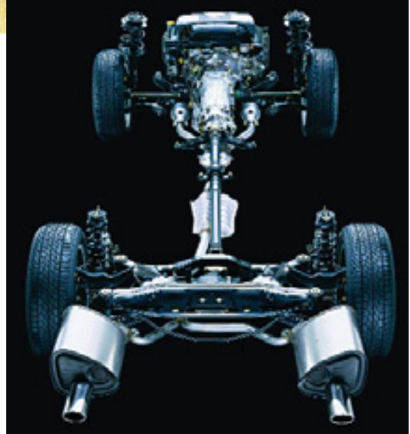
The lower center of gravity and balance of components are characteristics that give Symmetrical All-Wheel Drive superior stability and traction.
