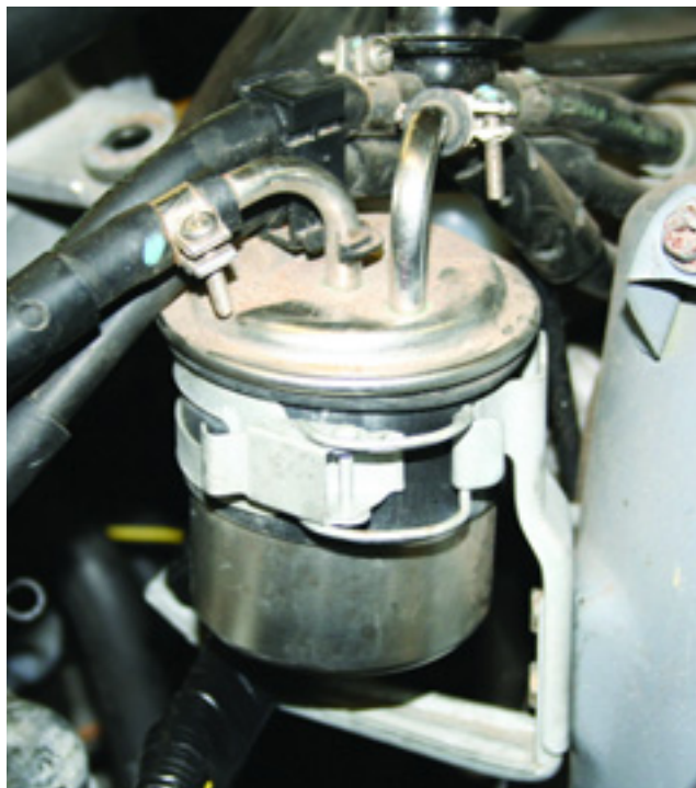
The underhood fuel filter is the last line of defense against contaminated fuel before it can reach the injectors. It should be replaced at 30,000 mile intervals.
