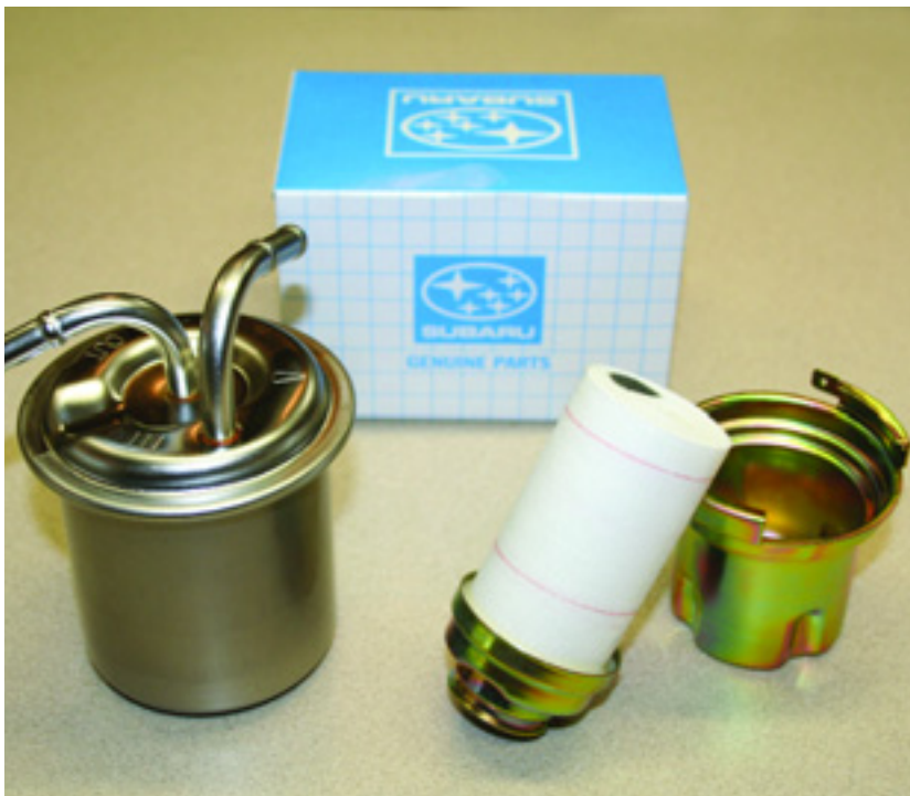
The underhood fuel filter, pictured on the left, has been used on many Subaru vehicles. In addition, the in-tank filter replacement cartridge on the right is located in the fuel pump assembly on recent models.
