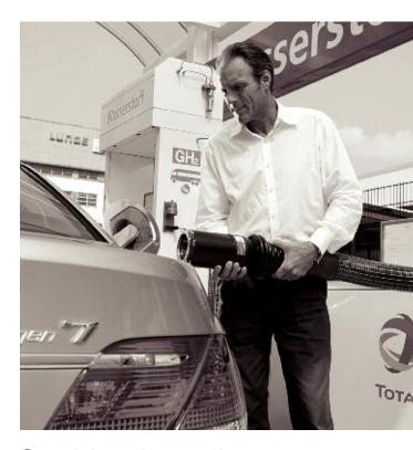
Special equipment is needed to refuel a hydrogen powered car, but the process is essentially the same as filling up any gasoline or diesel powered vehicle. In addition to a conventional gas tank, the BMW Hydrogen 7 car has a specially designed hydrogen storage tank. The hydrogen tank holds about 34-37 gallons of liquid hydrogen, stored at -250° C. (-418° F.). Dual walls, consisting of multiple
