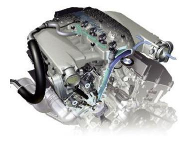
The 6-liter, 12-cylinder engine in the BMW Hydrogen 7 runs on either hydrogen or gasoline. Sophisticated control systems allow the driver to switch between fuels without any disruption in performance.
