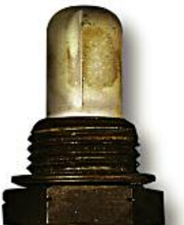
Fuel Contamination Burning a poor quality gasoline. Remind your customer that BMW recommends using only a Top Tier Detergent Gasoline with a minimum octane rating of 91. See www.toptiergas.com for more information.
