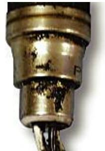
External Oil Leak An external oil leak has contaminated the sensor and its wiring.
