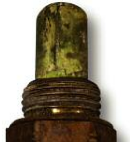
Coolant Contamination Coolant is leaking through the head/block seam, or the head casting itself and getting into the combustion chamber.
