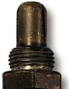
Oil Contamination Oil leaking into the combustion chamber or exhaust manifold.
