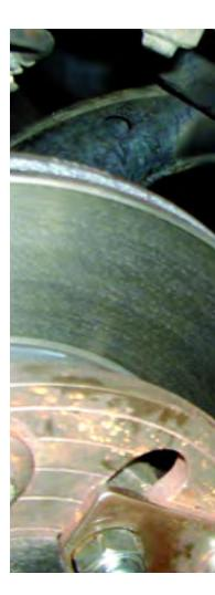
Although an on-car brake lathe can eliminate runout and DTV, you still haven't addressed the mounting error. So, there's apt to be trouble at the next reline.
