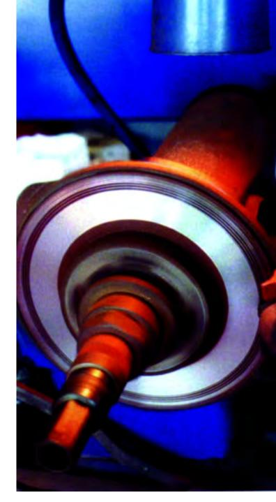
If you are turning rotors to eliminate pedal pulsation, you must make sure you mount them on the lathe arbor perfectly.
