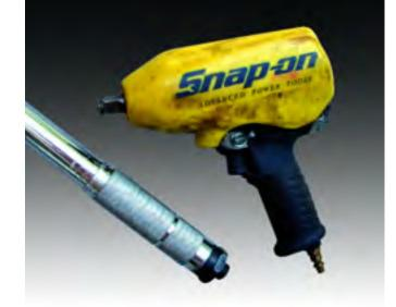
Always use a torque wrench for final lug tightening. Never use a 1/2 in. drive impact gun at all. Spin them down with a 3/8 in. drive tool on a low setting.
