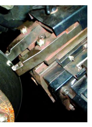
Yet, all rotors will eventually have to be replaced. So the solution is for techs to understand the causes and cures of runout rather than solely relying on the use of an on-car lathe every time the problem appears. Without such an understanding a tech would have to cut every brand new rotor on the car simply to correct for runout in the hub itself that gets "stacked" out to the rotor.
