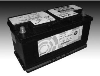
Advanced Glass Mat (AGM) batteries are less apt to gas and leak electrolyte than the traditional flooded-plate type, which reduces the potential for corrosion of components located nearby.
