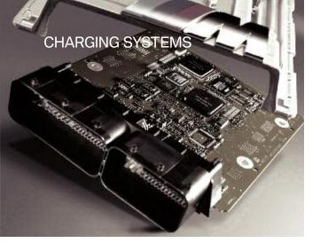
Engaging the "intelligence" of the ECM for the job of controlling alternator output makes for a much more efficient and effective charging system.
