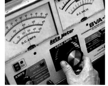
Even though charging system control is now handled by the ECM, the traditional VAT tester can still be used to force the alternator to produce at its maximum potential.
