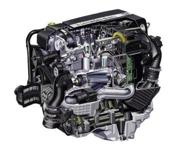
P2020 (P0172), P2046, P201C or P201A may be caused by a tear in the partial load vent hose at the connection to the crankcase. Air will bypass the mass air sensor - i.e. unmeasured air will enter the intake - causing the engine to run lean.
