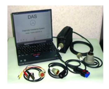
Mercedes-Benz developed DAS (also known as SDS), and here are all the components. The large black box to the right of the laptop is the Diagnostic Multiplexer. This multiplexer switches communication between control units on vehicles with the 38-pin and 16-pin diagnostic connectors.
