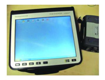
This is the Compact3, the tablet PC that contains the DAS and plugs into all the other peripherals.
