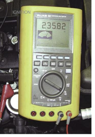
Here we are measuring the resistance of the shunt resistor. You must read 235 ohms. The red test lead is on the ground side, and the black lead on the coil side. You would need to reverse the leads to properly monitor the voltage drop as the coil fires.
