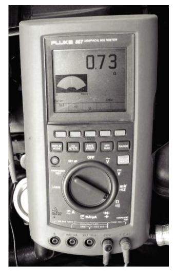
You do not have to remove the coil to determine its resistance. Backprobing the terminals will suffice. Remember, before '95 resistance of the primary winding is .45 ohms, and after '96 it's about .8 ohms.
