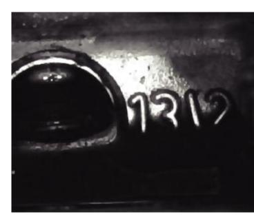
If you look down at the spark plug hole, you may see that it's filled with oil leaking from the valve covers. This can soften the boots and possibly allow the spark to arc to the cylinder head.
