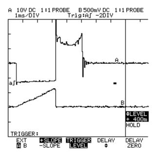
Watch the top pattern and you'll see the pull to ground, the inductive kick and the burn time. This shows that adequate spark took place. The lower waveform is the current pattern of the same coil. The low current probe was set to 100mV per amp. Just over one 500mV per division means over 5 amps are being produced. Compare to other cylinders, or previous test results.
