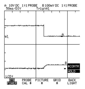
Here, the voltage control (upper trace) and amperage draw (lower trace) of a shift solenoid are being monitored. The resistance of these solenoids is about 30 ohms. In this case, the low current probe was set to put out 100mA per amp, so with the scope set to 100mA divisions we see just below .5 amp.
