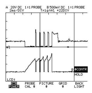
This is the MSD coil control. The top pattern is the voltage waveform. The lower waveform is the amperage draw. Each time you see the pattern rise and fall a spark is generated. This plug was fired five times at idle.
