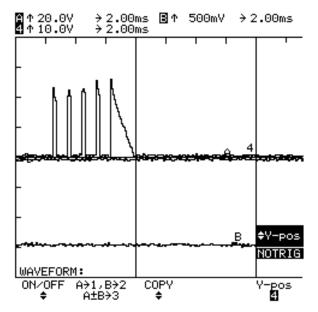
Here we are looking at the voltage kicks produced on the coil side of the shunt resistor for an MSD coil event. If these kicks are below two volts, the DME determines that there was a problem with combustion.
