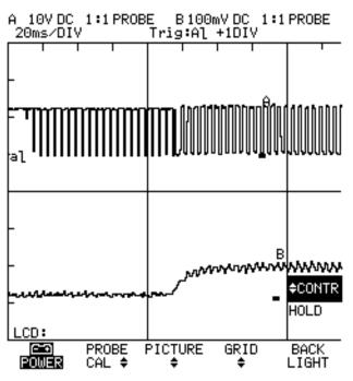
The voltage control (upper trace) and amperage draw (lower trace) of a pressure regulator solenoid are shown here. This solenoid is current-limited by the EGS unit. The solenoid is pulsed to ground, but there's no current draw. When the EGS activates the solenoid, it increases the duty cycle to ground, which in turn operates the solenoid.
