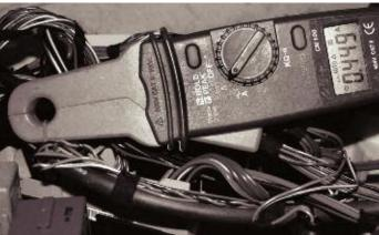
You can check the current draw with an inductive amp probe. In this case, one of the pressure regulator solenoids is being checked while it is activated. Here is the EGS control unit connector cover. Look for the locking tab. By pushing this tab out you can slide out the wiring connector, plug it back into the EGS and start testing.
