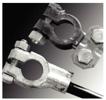
Emergency clamps are just that, but are often considered a permanent repair. Install a new cable and clamp assembly and you'll head off problems.
