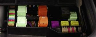
Minifuses don't always have to be removed and visually inspected. With power applied, you can touch DMM leads to the two tiny contacts on the face of most fuses to determine which show a 12V voltage drop, indicating they're blown, or use an inexpensive clip-on tester.
