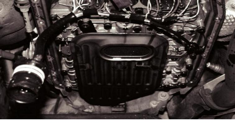
With the pan dropped and the connector removed, you can easily check the wiring harness inside the transmission. You can also check the solenoid resistance directly. The green solenoids are the shift solenoids and the black solenoids are the pressure regulator solenoids.
