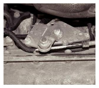
The gear selector switch is mounted on the side of the transmission on this ZF unit. There are a few technical service bulletins to look out for on this switch, so don't forget to check this first.
