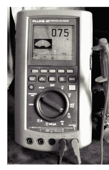
This is often the first test performed on a coil -the static test of primary winding resistance, measured across the two outside pins of the three-pin connector. Remember, just because a coil passes this test does not mean it is actually functioning.
