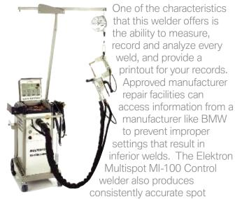
welds by using a microprocessor to control current and the welding time. It also allows the veteran welder to manually adjust controls, and will record this data.
