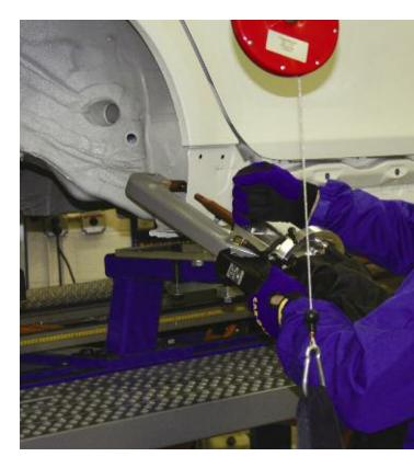
Today, squeeze-type resistant spot welders/resistance pressure spot welders must be used on BMW vehicles to assure a factory-like weld and avoid heat distortion.
