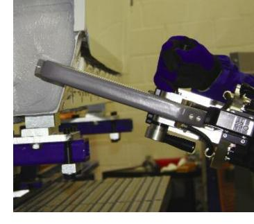
In all three recommended welders you will quickly see common themes: water cooling, programmability, and controllability so that vehicles are repaired in a way that assures passengers safety.
