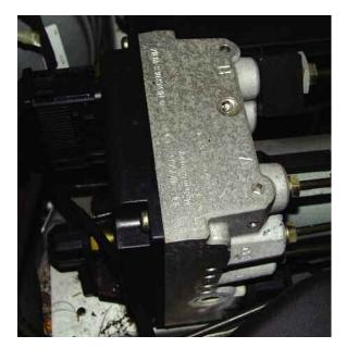
Although you see a control unit-type plug, it is only for the hydraulic solenoid assembly. This component houses the brake fluid control solenoids. The unit that controls the hydraulic assembly is mounted elsewhere.
