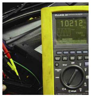
A more accurate way to test a wheel speed sensor is to check how much AC voltage it generates while spinning the wheel. Here, 1V AC is being produced by spinning the wheel by hand. Once again, this does not apply to Active Wheel Speed sensors.
