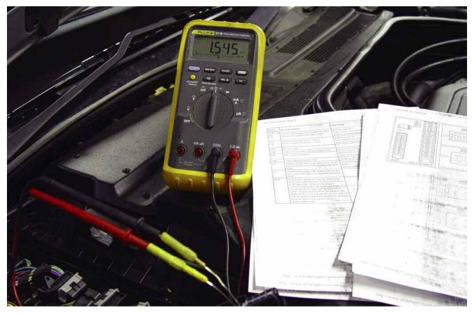
Since the control unit is so easy to get to, you can measure the resistance of the wheel speed sensors right from the connector. This not only checks the sensor resistance, but it also checks the wiring. This testing does not apply to Active Wheel Speed sensors.
