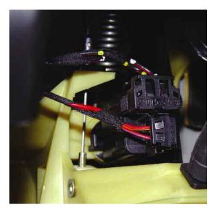
Here we have the dual output brake switch. One switch contact will be normally open (NO), and the other will be normally closed (NC). You can use the scan tool to watch this input, but a DMM will tell you if the switch contact is poor.
