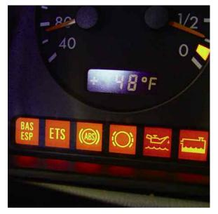
One way to determine what variations are on the system you are working on is to look at the warning lights during a bulb check. You can see that this vehicle has BAS, ESP (which means it has ASR also) and ETS. If these lights stay on with the engine running, you definitely have a fault in the system.
