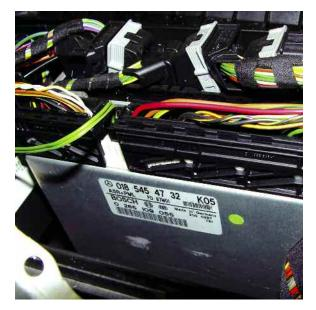
This control unit is one of many on the powertrain CAN. This ASR control unit has traction control, but in this '97 S320 does not have ESP. Notice how easy it is to perform electrical testing at this unit. Under "Diagnostics," you're given the pin voltages to test for.
