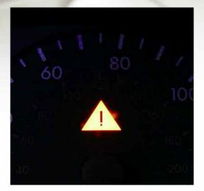
The ASR warning light will illuminate when the system is commanded not to function, either through the "ASR Off" switch, or if there is a fault in the system. When the light comes on while driving, it does not mean there is a DTC in the system. It means there is a problem with traction at that time.
