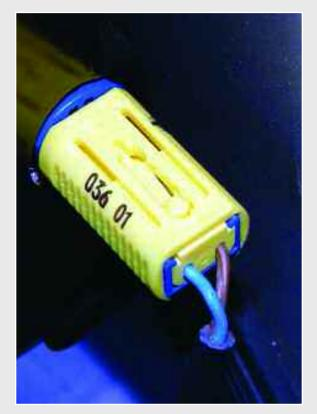
Yellow connectors and harness tape indicate that this is airbag system wiring. This is a two-wire squib for the door-mounted airbag. If you had a fault code for this airbag, you would open this connector and measure resistance between it and the SRS control unit.
