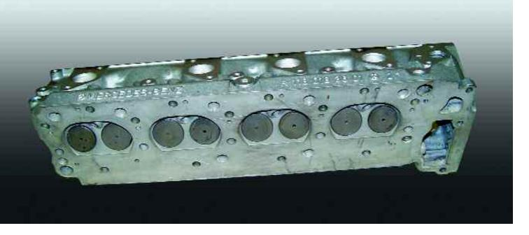
After cleaning, measure the surface straightness of the cylinder head mating surface. In this case it was necessary to mill the cylinder head, and the head thickness was sufficient to do so. This creates a near ideal surface for the head gasket to seal against.
