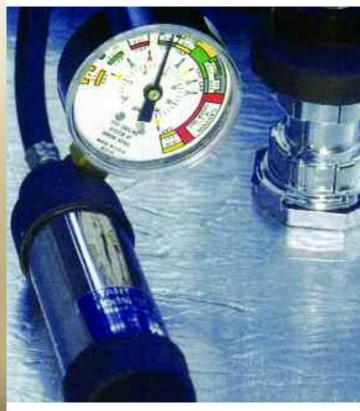
Pressure testing the cooling system may force coolant through a leaking cylinder head gasket. With a boroscope you can see into the cylinder and observe if there is any coolant seepage.
