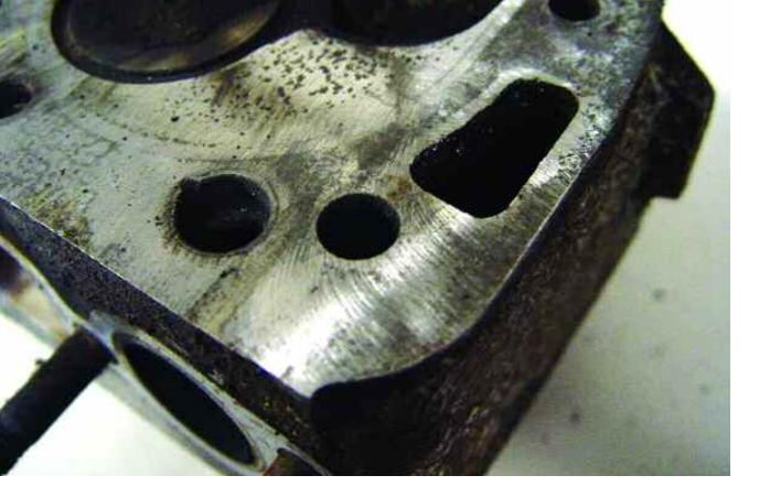
Here we can see the swirl marks left by surface conditioning discs. If you stay in one portion of the cylinder head too long you can create a dip that the head gasket may not be able to seal. So, clean the cylinder head by hand using suitable scrapers.
