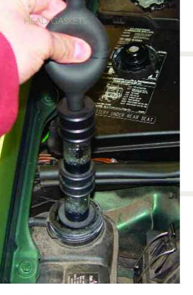
Using a combustion gas leak detector will allow you to determine if there's a leak between the combustion chamber and the cooling system. Don't forget to drain some coolant out of the system to build up sufficient combustion gas.
